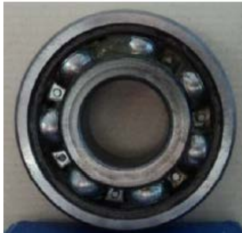
Figure 4 ZMCO-6304 Bearing in healthy condition
